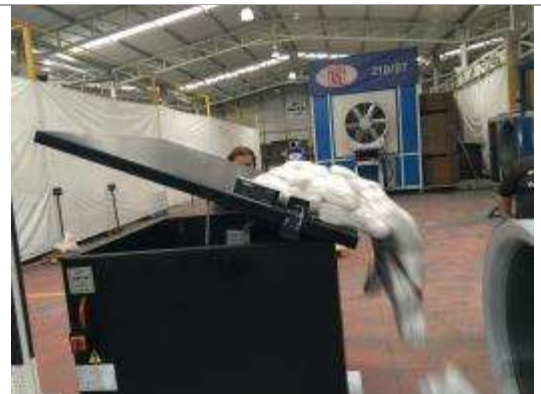
Description: Damper tested 3 times with loaded 102 kg. Damper position was reached at fire operating position less than 30 second each time after Snow load test.
