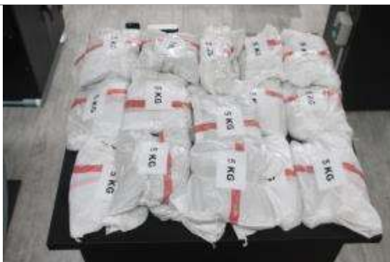
Description: The bags were uniformly distributed over the external surface of Cabinet Roof Type Axial Smoke Exhaust Fan. Snow load test with 102 kg during 10 minutes.
