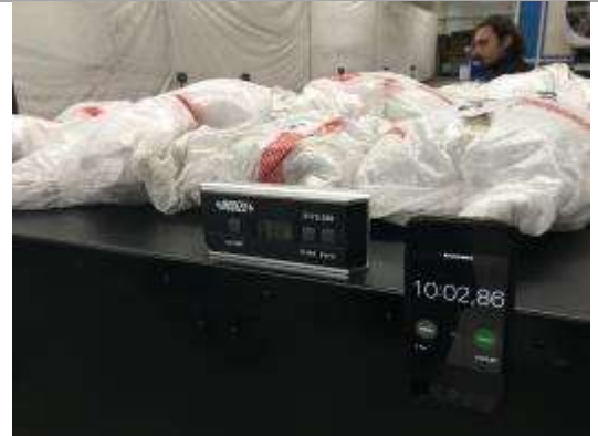
Description: Wind load test with 60 kg during 10 minutes
