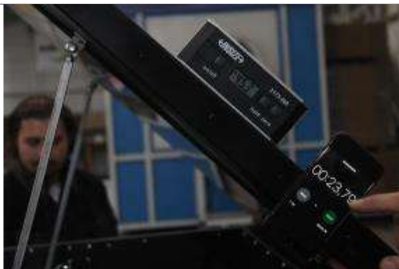
Description: Damper tested 1 time with unloaded. Damper position was reached at fire operating position less than 30 second after Wind load test.
