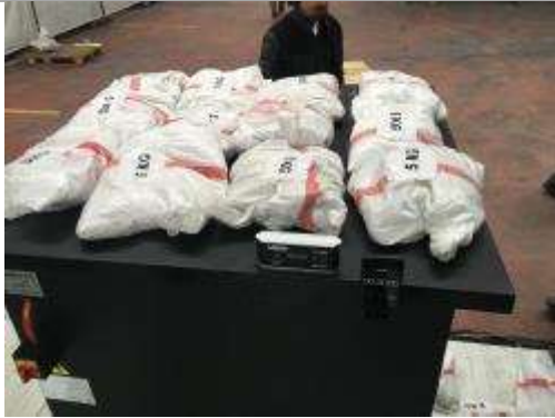
Description: The bags were uniformly distributed over the external surface of Cabinet Roof Type Axial Smoke Exhaust Fan. Wind load test with 60 kg during 10 minutes
