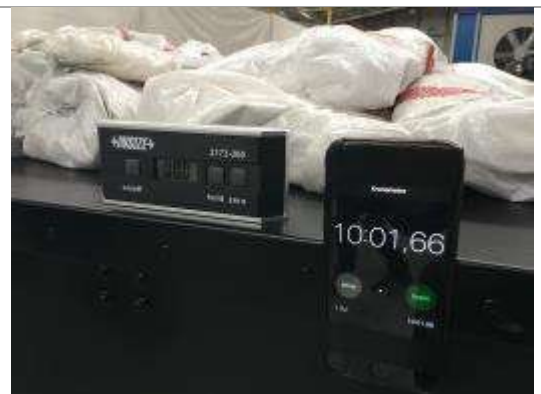
Description: Snow load test with 102 kg during 10 minutes
