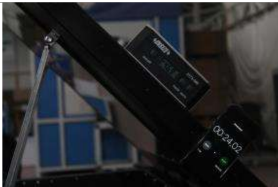
Description: Damper tested 1 time with unloaded. Damper position was reached at fire operating position less than 30 second after Snow load test.
