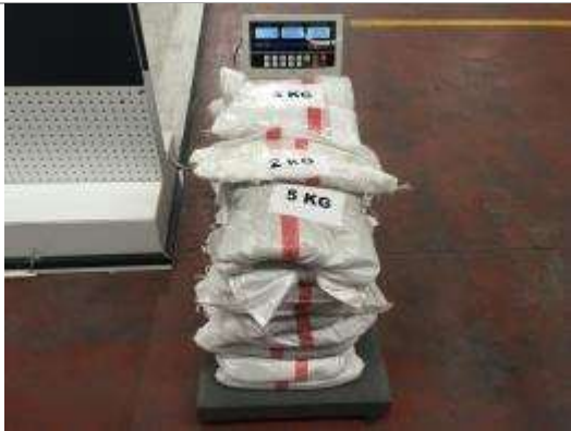
Description: Weighing for 102 kg. Bags were containing 5 kg of solid particles
