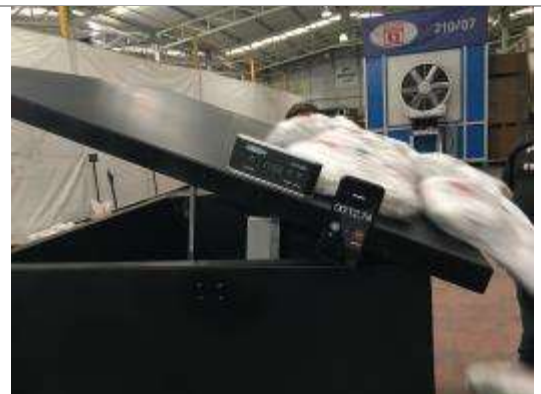
Description: Damper tested 3 times with loaded 60 kg. Damper position was reached at fire operating position less than 30 second each time after Snow load test.
