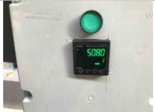
Description: Counter at the end of the open-close test
