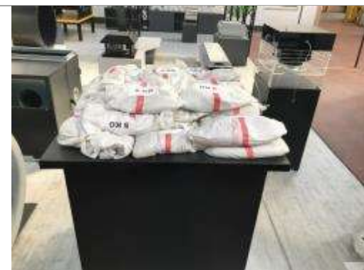
Description: The bags were uniformly distributed over the external surface of Cabinet Roof Type Axial Smoke Exhaust Fan. Combination of wind load and snow load test with 162 kg during 10 minutes.
