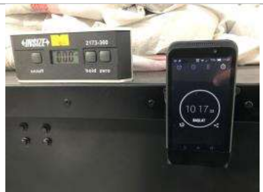
Description: Damper tested 1 time with unloaded. Damper position was reached at fire operating position less than 30 second after 10 minutes.
