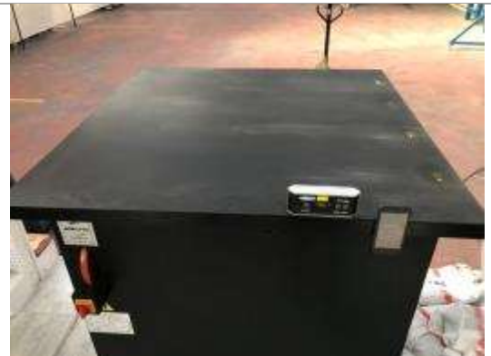
Description: It was not observed any deformation on the Cabinet Roof Type Axial Smoke Exhaust Fan After Combination of Snow load test and Wind load test and open-close test
