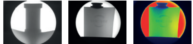
Fan blades are tested against discontinuity by the radiography method
